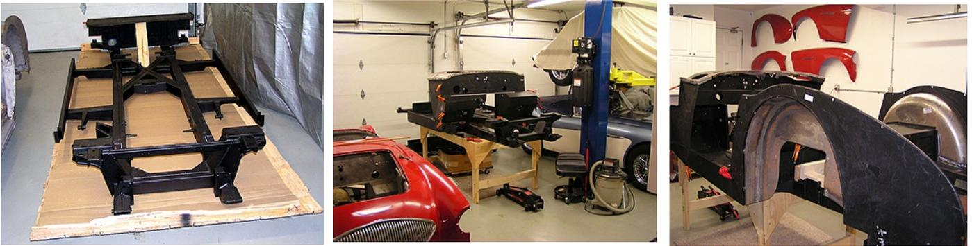
The welding of rear bumper outriggers, emergency brake supports, front motor mounts, firewall and radiator supports, etc. is now complete. These along with the temporary affixing of other tub components is also complete. The last photo illustrates the rear shroud in place, albeit temporary, this tells me that the progress is in the right direction. My current problem is some sheet metal welding difficulties with the 19 gauge tub pieces. For the present -cheers!
