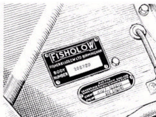
The Chassis Number is stamped on a plate secured to the right-hand side of the firewall.
